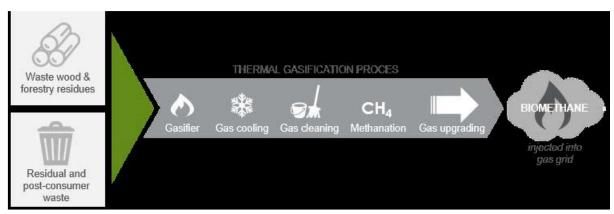
Figure 4: Schematic overview of the thermal gasification process
