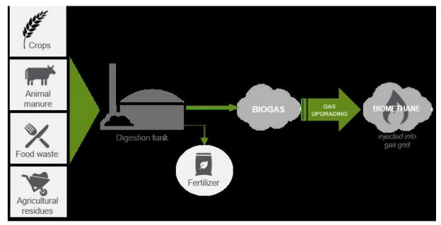
Figure 3: Schematic overview of the anaerobic digestion process.
