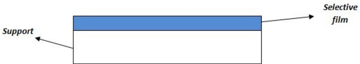
ure 2 – Composite membrane architecture
