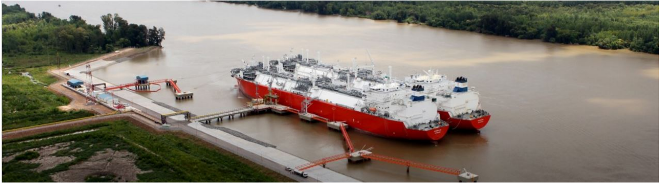
Fig. 4 – FSRU vessel for LNG transportation and regasification
