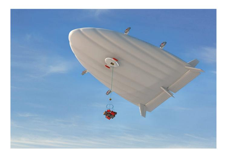
This airship, called the HA2t, can lift 2 tons into remote areas, and can be shipped in a standard cargo container. (Source: Total)
