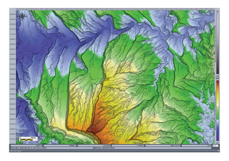
LiDAR data are used to map the contours of the survey area during the planning process. Source: Total.
