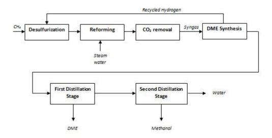
In the two steps (indirect) process, the methanol formation from syngas and the DME production from methanol are supported in two separated reactors, where the specific catalysts (copper-based for the first, silica-alumina for the second) are packed. The figure illustrates the block diagram of this architecture.
