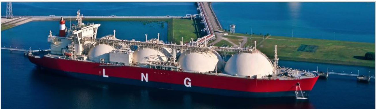
Fig. 3 – FSU vessel for LNG transportation
