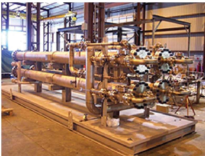
Figure 5 – SourSep™ MTR installation for the removal of H 2 S.
