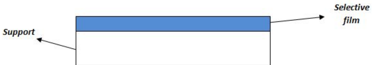
ure 2 – Composite membrane architecture
