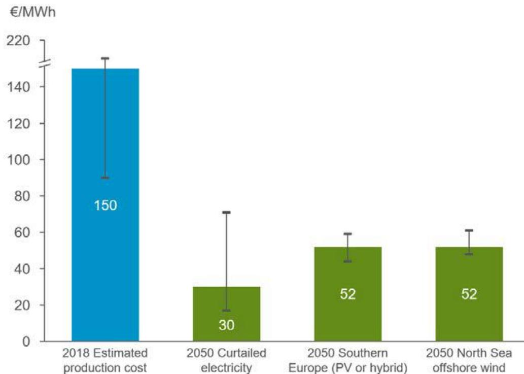
Figure 6: Green hydrogen production cost estimation for 2018 and 2050.
