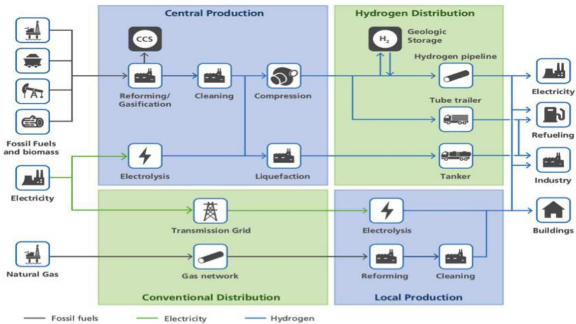
Figure 1: Hydrogen sources, production, distribution and applications.
