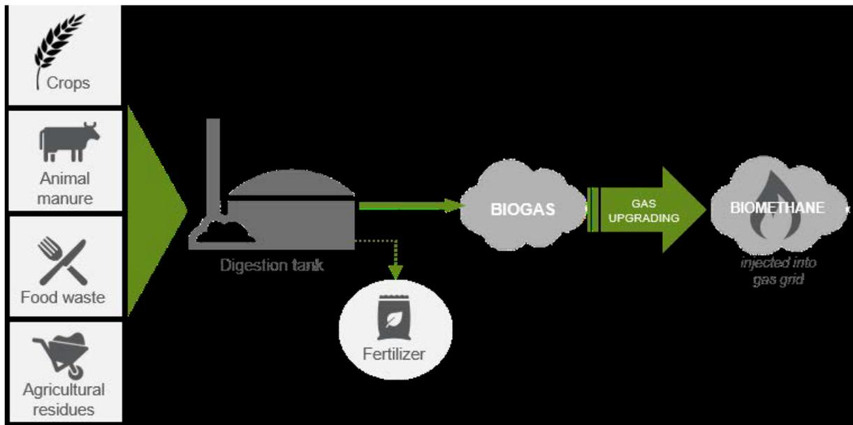
Figure 3: Schematic overview of the anaerobic digestion process.
