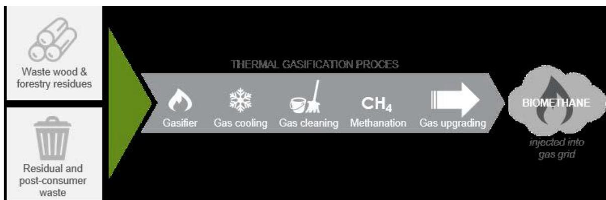
Figure 4: Schematic overview of the thermal gasification process
