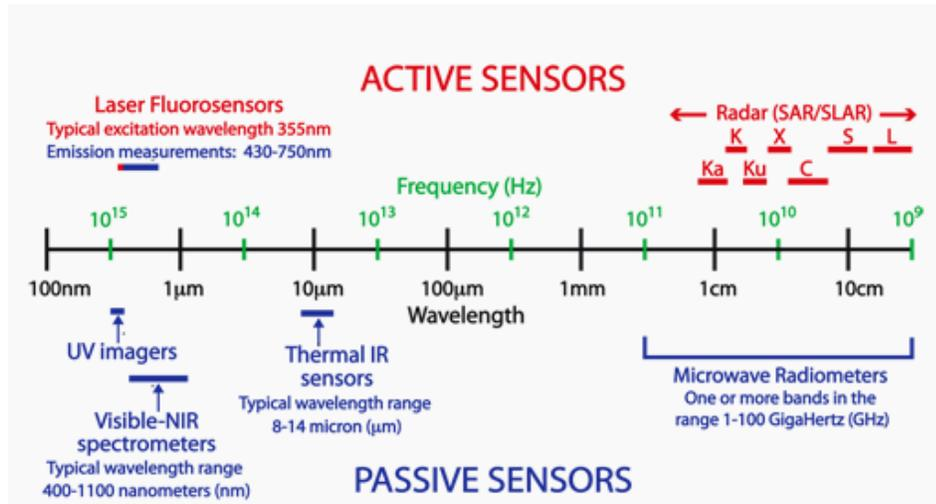
Figure 3-3-1 Remote sensing devices classification<sup>11</sup>.
