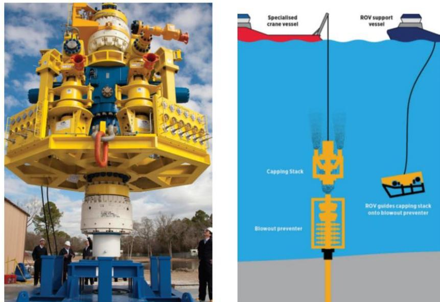
Figure 2-1 Capping stack system (left);Capping stack installation (right)<sup>9</sup>.
