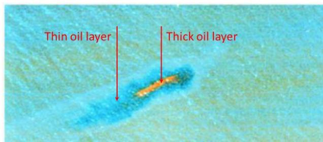
Figure 3-3 Infrared image of oil spill<sup>15</sup>.
