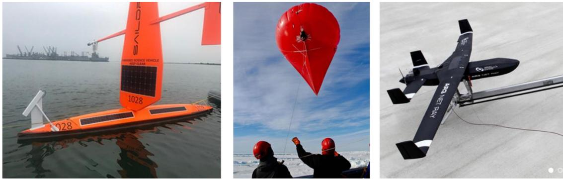
Figure 3-3-2 Salidrone unmanned surface vehicle<sup>12</sup> (left); aerial observation spill response balloon<sup>13</sup> (center), unmanned fixed wing aircraft<sup>14</sup> (right).
