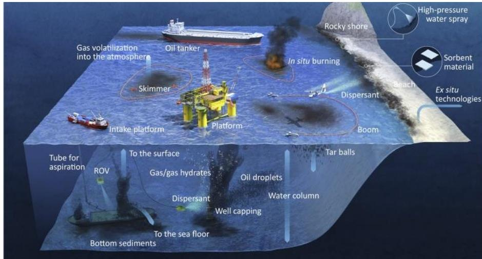
Figure 1-2 A visual overview of all the oil spill response techniques<sup>6</sup>.
