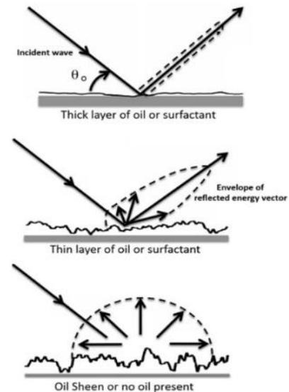
Figure 3-4 The variation of radar backscatter due to oil or surfactant on the sea surface<sup>15</sup>.
