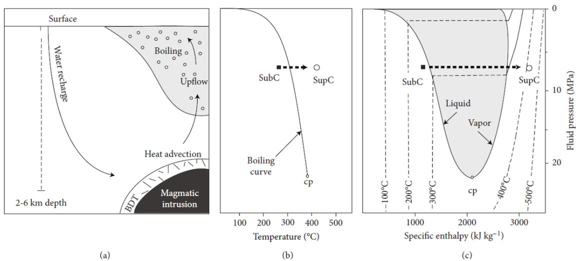
**Figure 3 : Main characteristics of a volcanic geothermal system. (a) Conceptual model showing fluid flow paths, the brittle-ductile transition (BDT) between the magmatic heat source and the circulating geothermal fluid, and depressurization boiling near the surface. (b) The boiling curve of water. (c) The phase diagram of water showing pressure, specific enthalpy, and temperature relations. Also shown are the subcritical (SubC) to supercritical (SupC) conditions <sup>10</sup>**
