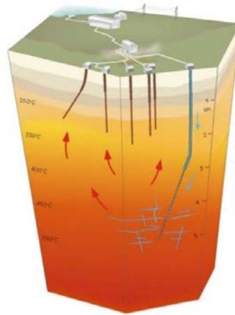
Figure 6 A conceptual model showing the EGS (Enhanced geothermal system) system in the Reykjanes field<sup>17</sup>
