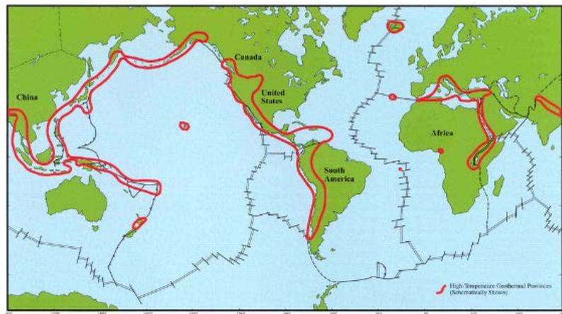
Figure 4 Outlined in red are the worldwide zones where very high enthalpy, possibly supercritical geothermal resources could exist at drillable depths. <sup>13</sup>
