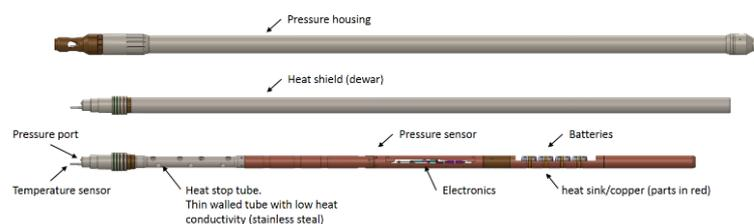
**Figure 17 (Top)The complete tool with pressure housing. Temperature sensor and pressure port to the left (nose) and connection for the slick line wire to the right. (Middle)Pressure shield and nose protector removed. Picture show the nose of the tool and the heatshield. (Bottom) Heat shield removed. Pictures how the inner parts of the tool. Electronics located in the middle of the tool <sup>49</sup>**
