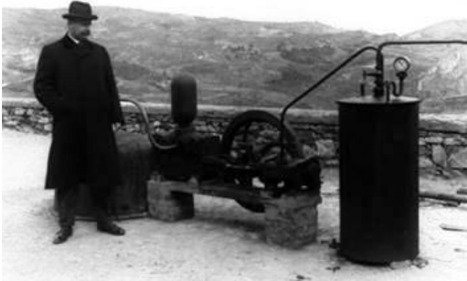
Fig.3 – Lardareello 1904: Prince Piero Ginori-Conti with his apparatus that converted geothermal to electrical energy for the first time in history. (From: UGI 2010)
