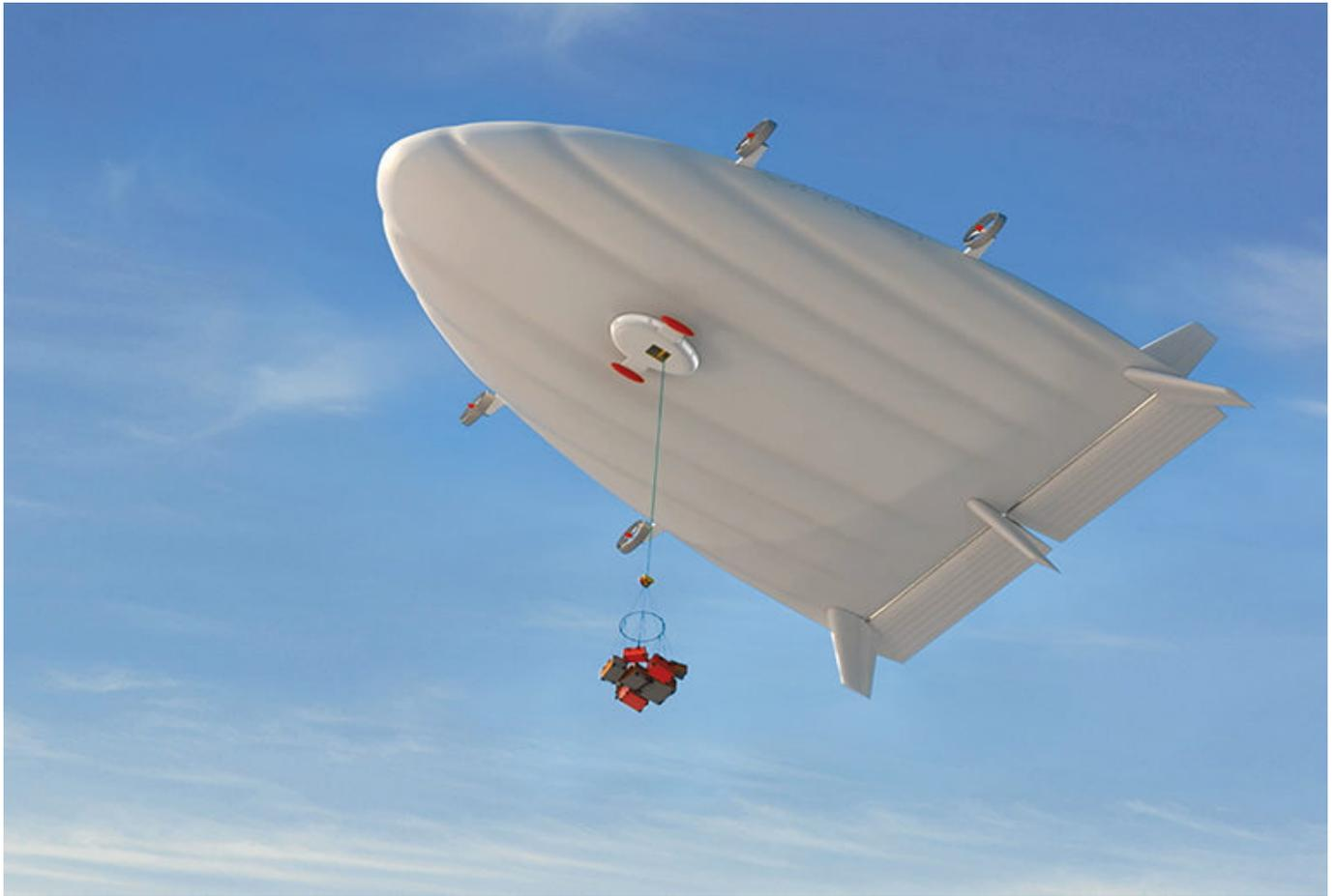
*This airship, called the HA2t, can lift 2 tons into remote areas, and can be shipped in a standard cargo container. (Source: Total)*
