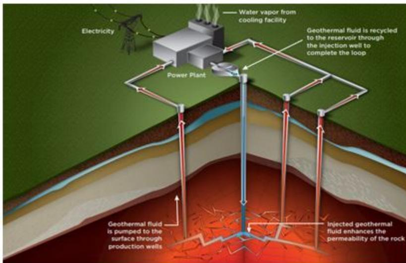
**Fig. 2 Enhanced Geothermal System illustration (U.S. Department of Energy)**
